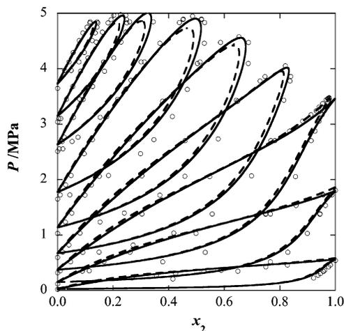
**Figure 9.** Constant temperature  $p$ - $x$  slices for the methane (1) + nitrogen (2) binary mixture at 95, 113, 127.59, 138.44, 149.82, 160.93, 172.04, 177.59, and 183.15 K (from bottom to top). The solid lines represent predictions from the quadrupolar SAFT-VR equation with  $k_{ij} = 0.0395$ , and the dashed line represents predictions from the original SAFT-VR approach with  $k_{ij} = 0.118$  and  $\gamma_{ij} = -0.028$ . The symbols are experimental data taken from refs 71, 72.
