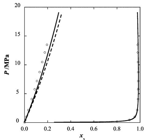
**Figure 4.** Constant temperature  $p$ - $x$  slices of the phase diagram for the butane (1) + nitrogen (2) binary mixture at 250 K. The continuous curves correspond to predictions from the quadrupolar SAFT-VR approach, and the dashed curves, predictions from the original SAFT-VR equation. The circles represent the experimental results taken from ref 73.
