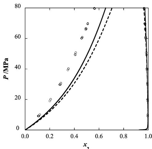
**Figure 6.** Constant temperature  $p$ - $x$  slices of the phase diagram for the heptane (1) + nitrogen (2) binary mixture at 305.4 K. The continuous curves correspond to predictions from the quadrupolar SAFT-VR approach, and the dashed curves, predictions from the original SAFT-VR equation. The circles are experimental results taken from ref 75.
