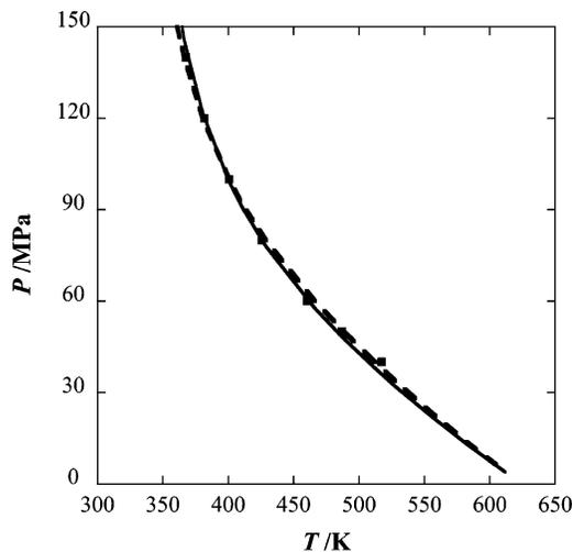
**Figure 11.**  $p$ - $T$  projection of the critical line for the decane (1) + nitrogen (2) binary mixture. The continuous curves correspond to predictions from the quadrupolar SAFT-VR equation with  $k_{ij} = 0.285$  and  $\gamma_{ij} = -0.089$ , and the dashed curves, predictions from the original SAFT-VR equation with  $k_{ij} = 0.289$  and  $\gamma_{ij} = -0.089$ . The symbols are experimental data taken from ref 84.
