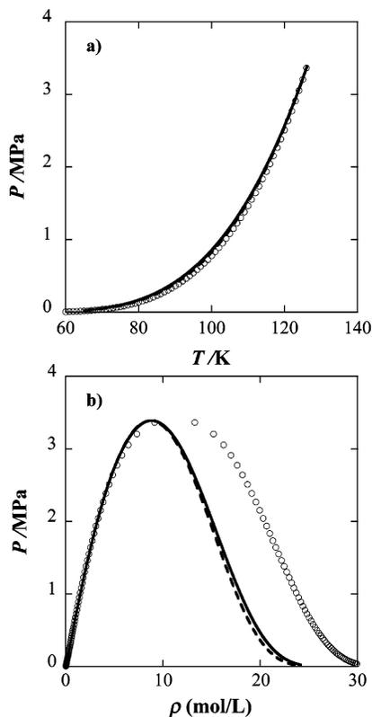
**Figure 2.** (a) Vapor pressure and (b) coexisting densities of nitrogen compared with theoretical results using rescaled parameters. Solid line represents predictions from the quadrupolar SAFT-VR approach, dashed line, results from the original SAFT-VR equation, and circles, the experimental data taken from ref 70.
