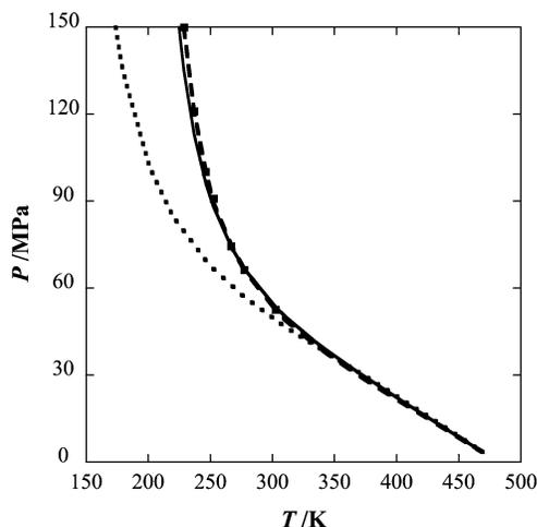
**Figure 10.**  $p$ - $T$  projection of the critical line for the pentane (1) + nitrogen (2) binary mixture. The continuous curves correspond to predictions from the quadrupolar SAFT-VR approach with  $k_{ij} = 0.0395$ , the dashed curves, predictions from the original SAFT-VR equation with  $k_{ij} = 0.216$  and  $\gamma_{ij} = -0.066$ , and the dotted curves, the original SAFT-VR with  $k_{ij} = 0.118$  and  $\gamma_{ij} = -0.028$ . The symbols are experimental data taken from ref 77.
