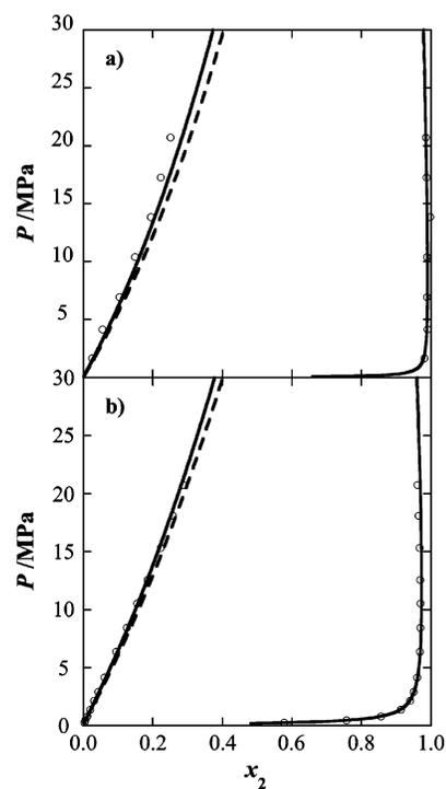
**Figure 5.** Constant temperature  $p$ - $x$  slices of the phase diagram for the pentane (1) + nitrogen (2) binary mixture at 277.43 and 310.7 K (from top to bottom). The continuous curves correspond to predictions from the quadrupolar SAFT-VR approach, and the dashed curves, predictions from the original SAFT-VR equation. The circles represent experimental data taken from ref 74.
