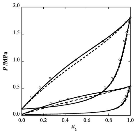
**Figure 3.** Constant temperature  $p$ - $x$  slices of the phase diagram for the methane (1) + nitrogen (2) binary mixture at 95 and 113.7 K (from bottom to top). The continuous curves correspond to predictions from the quadrupolar SAFT-VR equation, and the dashed curves, from the original SAFT-VR approach. The circles represent the experimental results taken from refs 71 and 72.
