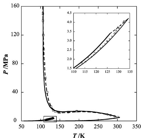
**Figure 7.**  $p$ - $T$  projection of the ethane (1) + nitrogen (2) phase diagram. The continuous curves correspond to predictions from the quadrupolar SAFT-VR approach, and the dashed curves, predictions from the original SAFT-VR equation. The symbols represent experimental data taken from refs 76–80.
