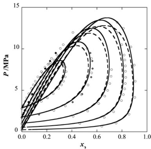
**Figure 8.** Constant temperature  $p$ - $x$  slices for the ethane (1) + nitrogen (2) binary mixture at 200 K, 220 K, 240 K, 260 K, and 280 K (from left to right). The solid lines represent predictions from the quadrupolar SAFT-VR approach with  $k_{ij} = 0.0395$  and the dashed line predictions from the original SAFT-VR equation with  $k_{ij} = 0.118$  and  $\gamma_{ij} = -0.028$ . The symbols are experimental data from refs 79, 81–83.
