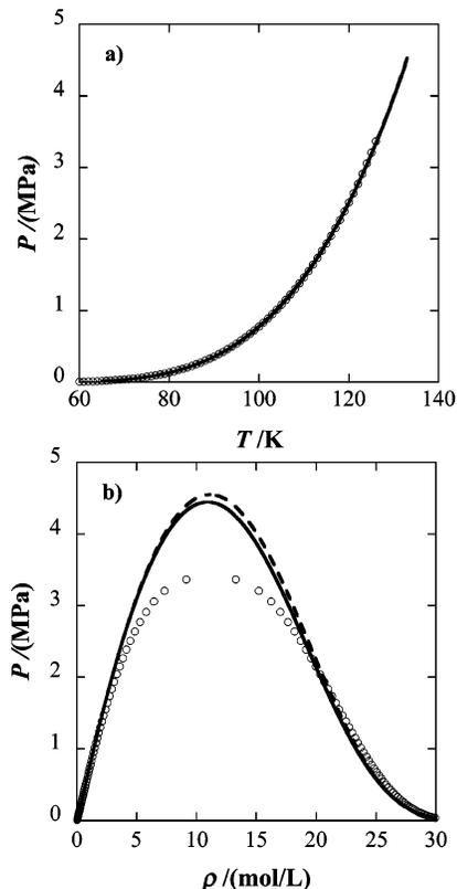
**Figure 1.** (a) Vapor pressure and (b) coexisting densities for nitrogen. Solid line represents predictions from the quadrupolar SAFT-VR approach, dashed line, results from the original SAFT-VR equation, and circles, the experimental data taken from ref 70.
