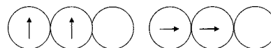
FIG. 13. Schematic illustrating the triatomic molecular model used to describe a chain fluid with dipole moments embedded in the center of the first two segments. Segments are labeled 1–3 from left to right.
