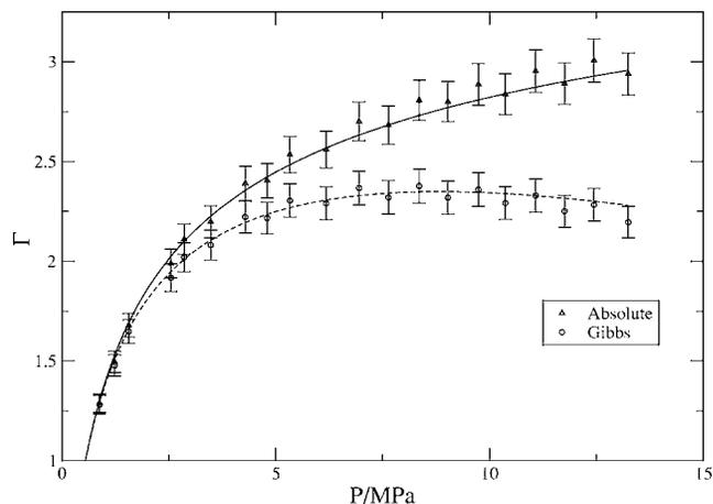
FIG. 3. Adsorption isotherms for methane adsorbed on dry activated carbon at 318.2 K. Gibbs and absolute adsorption isotherms are reported scaled with their respective values at 0.55 MPa. Theoretical correlations are represented as lines and the experimental data (Ref. 48) as symbols.
