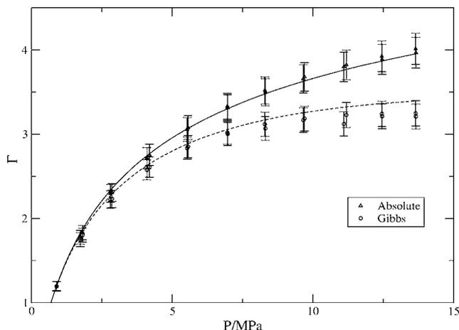
FIG. 4. Adsorption isotherms for nitrogen adsorbed on dry activated carbon at 318.2 K. Gibbs and absolute adsorption isotherms are reported scaled with their respective values at 0.69 MPa. Theoretical correlations are represented as lines and the experimental data (Ref. 48) as symbols.
