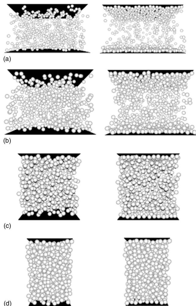
FIG. 2. Snapshots of configurations from simulations reported in Fig. 1. Left-hand-side images correspond to  $\epsilon^* = \epsilon_w / \epsilon = 2.0$  with bulk fluid packing fractions  $\eta$  given as (a) 0.0329, (b) 0.0606, (c) 0.1583, and (d) 0.3789. Right-hand-side images correspond to  $\epsilon^* = 8.0$  with  $\eta$ : (a) 0.0179, (b) 0.0400, (c) 0.1289, and (d) 0.3737.
