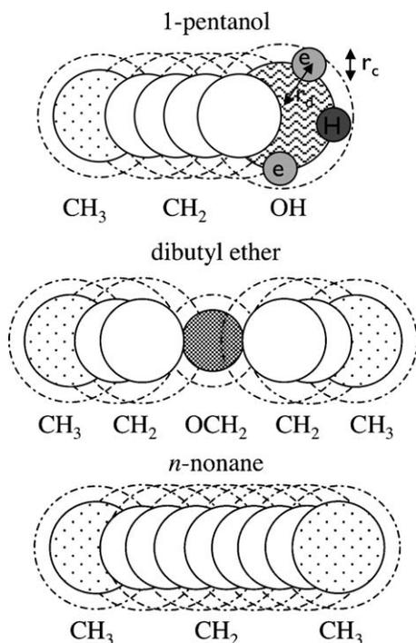
**Fig. 1.** Schematic representation of the molecular model used to describe 1-pentanol, dibutyl ether, and *n*-nonane molecules in the GC-SAFT-VR approach.
